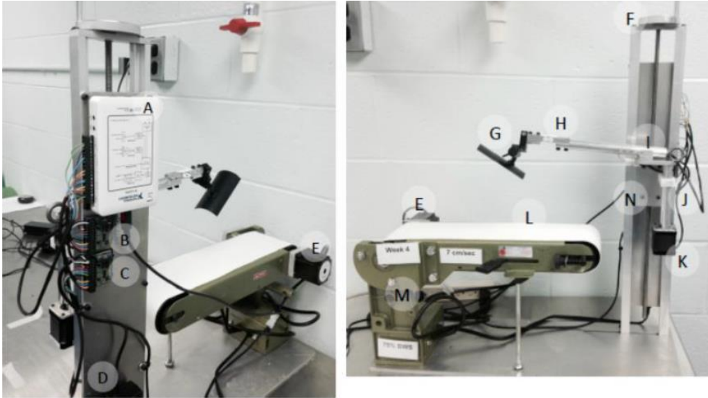
Figure 26. Images of the custom built body weight support treadmill. (A) National Instruments myDAQ system, paired with LabVIEW VI operating system; (B) Treadmill motor controller connected to myDAQ, controlling motor to drive treadmill; (C) Tensioning motor controller connected to myDAQ, controlling tension in spring; (D) Power supply cord, connects to outlet; (E) Treadmill motor; (F) Adjustment knob to lower or raise body weight support arm; (G) Animal attachment plate; (H) Load cell, measuring weight animal is subjected to; (I) Load cell amplification circuit, amplifying load cell signal before processed by myDAQ; (J) Tension spring, proving assistance to animal; (K) Spring tension motor, changes tension of spring via tension motor controller; (L) Treadmill belt; (M) Base of treadmill; (N) Body weight support carriage, attached to the adjustment knob and moves spring and load cell
