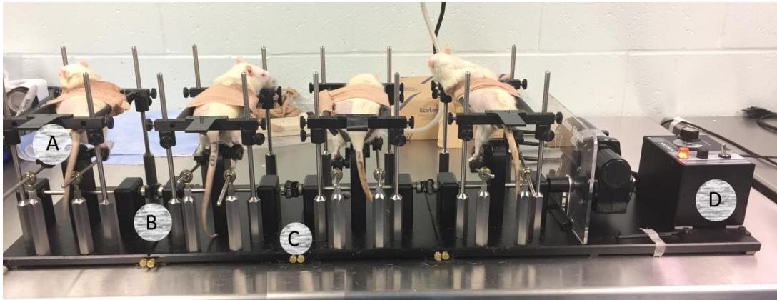
Figure 28: Image of bike set up. (A) Rectangular frame for holding rat, screwed into place by adjustable knobs attached to vertical metal rods; (B) Base frame, supporting rotating connectors and pedals; (C) Base connectors held in place by metal screws; (D) DC Motor with adjustable speed control, powers pedals
