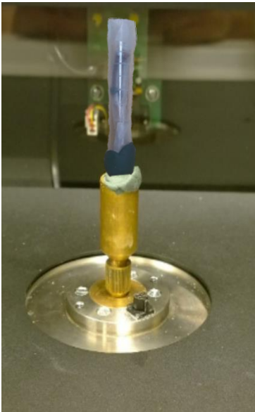
Figure 29. Rat tibia in para-film wrapped tube on top of metal brass stage prepared for scanning
